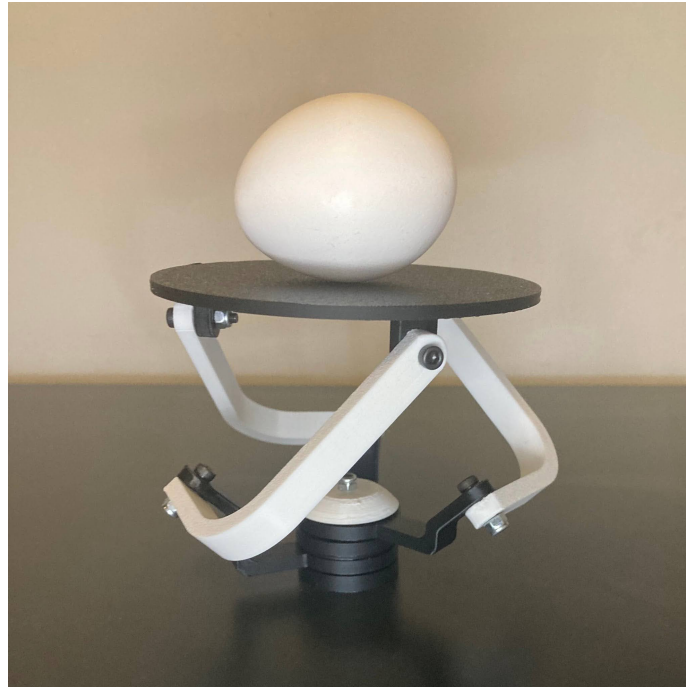
Figure 35: Final 3D-Printed and Assembled Spherical Parallel Manipulator
