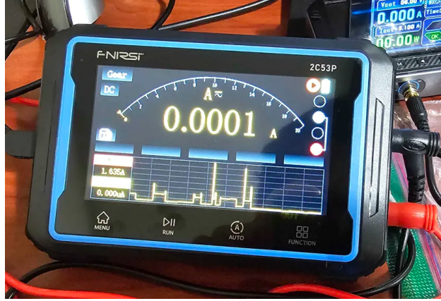
Figure 10: Current spike detected by the ammeter
